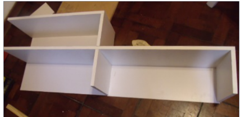
4. I made the remaining two shelves each 8" high. I set the length of the successive shelves to match the rise of the staircase behind them. I used screws to assemble, and drilled pilot holes, which made assembly easy.
